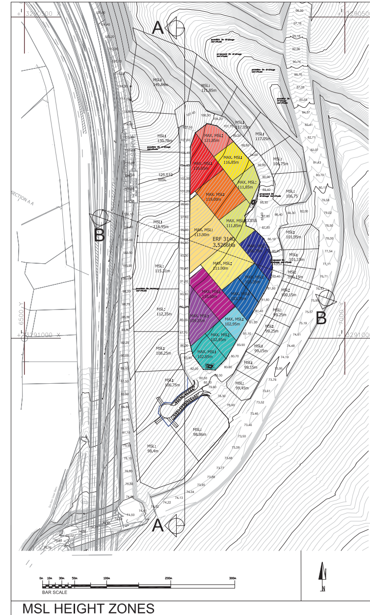
Figure 3:2 Precinct 3 Contour Plan and Mean Sea Level Height Specification - for msl benchmarks refer to surveyor's drawings
